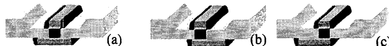
Figure 3. Asymmetrical DG with 50 nm front gate and 100 nm back gate. Back gate can be centred (a), shifted towards the drain (b), or towards the source (c).
