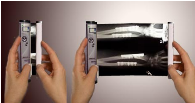
Figure 1 An artist's rendition of a flexible and rollable display which can be rolled out from a compact pen-sized form for viewing.
