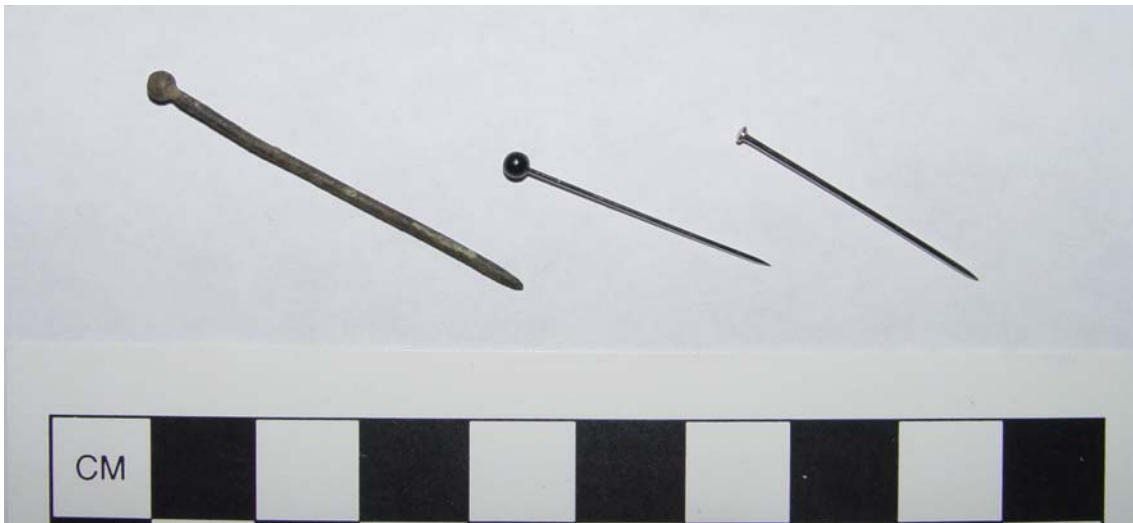
Figure 13.5: Comparison of FBC Straight Pin (left) with Present Day Straight Pins (center & right)
