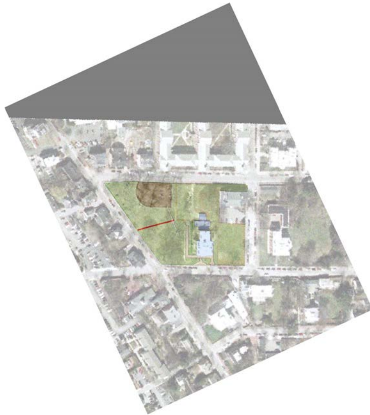
Satellite view with GIS overlay of the John Brown House property with baseline (red) and property boundaries marked as measured by the Total Station survey of November 2008. The datum is a point on the eastern (right) terminus of the baseline (map Brad Sekedat).
