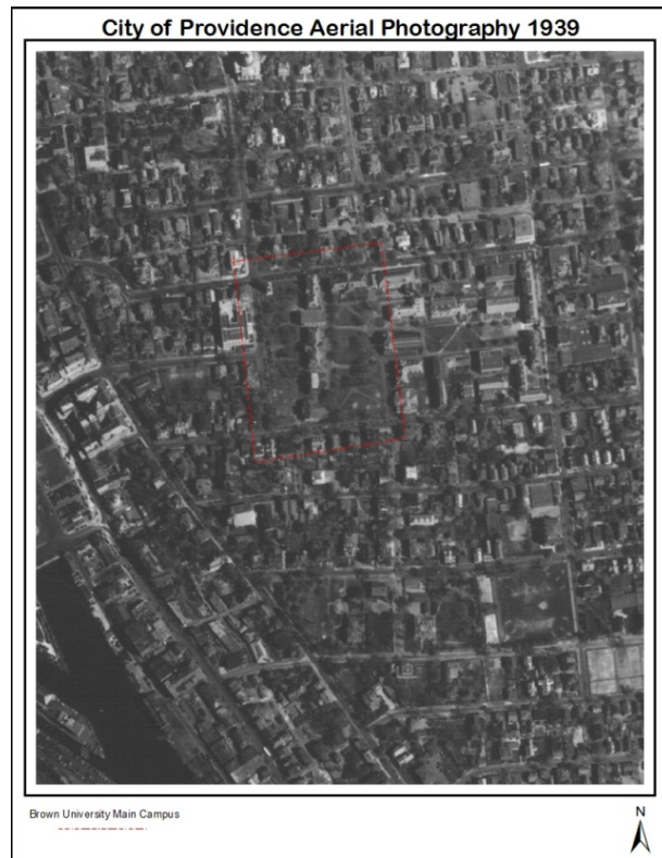
FIGURE 5.15 1939 Aerial image of Providence on an unknown coordinate system and therefore cannot be projected with other datasets. This is a helpful visual aid but it really emphasizes that a data user needs to fully understand what they’re looking at in order for the data to be used properly. (Map courtesy of RIGIS 2002)
