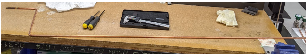
Figure 6. Copper-methanol prototype thermosyphon made by ACT.
