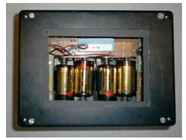
A cutout is made in the bottom of the enclosure for easy access to the batteries. The battery compartment is covered with black lexan sheet (not shown).
