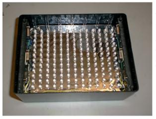
The LED array and the electronics fit inside the box and rests on standoffs. Roller switches mounted on a bracket on the side of the box detect when an object is place on the blicket box. A paper diffuser (not shown) is placed in between the LEDs and the top of the box to provide a more uniform lighting.
