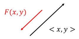
$$\|\mathbf{F}(x,y)\| = \sqrt{\left(-\frac{x}{\sqrt{x^2 + y^2}}\right)^2 + \left(-\frac{y}{\sqrt{x^2 + y^2}}\right)^2} = \sqrt{\frac{x^2 + y^2}{x^2 + y^2}} = \sqrt{1} = 1$$
