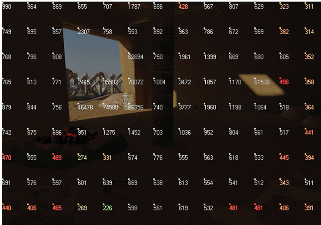
Figure 6. Lighting analysis of the interior of Building 1 with image overlay effect on 20 March 2013, 9am (image © Constantinos Papadopoulos).
