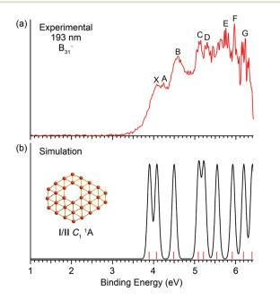
Fig. 1 Photoelectron spectrum of  $B_{31}^{-}$  at 193 nm (a) compared with the simulated spectra of the lowest-lying isomers of  $B_{31}^-$  ( $C_1$ , I and II) (b) at the TD-PBE0/6-311+G(d) level. The simulated spectra were obtained by fitting the calculated VDEs (vertical red bars) with unit-area Gaussian functions of 0.05 eV half-width.
