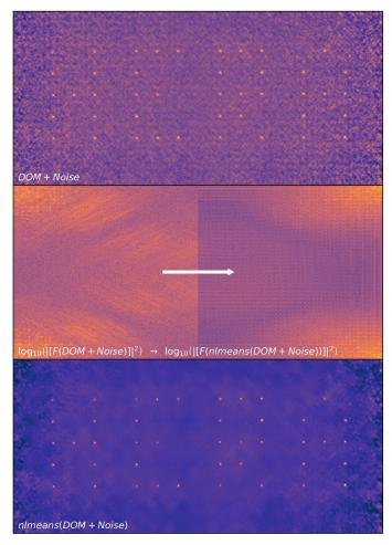
**Fig. 8.** Fourier filter schematic for Figure 4 with additional Gaussian noise added. See annotations; *F* represents a 2D Fourier transform. (The arrow shows how the original power spectrum is modified—this is a stand-in intermediary for the result from skimage non-local means, which is similar to a full covariance matrix filter.)
