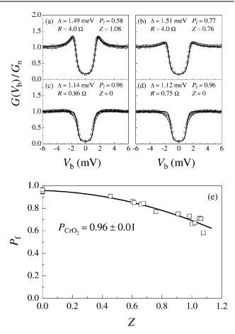
FIG. 4. (a)–(d) Measured  $G(V_b)/G_n$  versus  $V_b$  of Pb/CrO<sub>2</sub> point contacts at T = 1.85 K for different contact resistances (open circles). The solid lines are fits to the data with the BTK model resulting in  $P_f$ , Z, and  $\Delta$  as indicated in the figure. (e) Fitted polarization  $P_f$  as a function of Z. The solid line is a polynomial fit of the data to extract the spin polarization  $P_{CrO_2} = 0.96 \pm 0.01$  in the limit of Z = 0.
