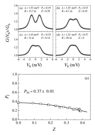
FIG. 3. (a)–(d) Measured  $G(V_b)/G_n$  versus  $V_b$  of Nb/Ni point contacts at T = 4.2 K for different contact resistances (open circles). The solid lines are fits to the data with the BTK model resulting in  $P_f$ , Z, and  $\Delta$  as indicated in the figure. (e) Fitted polarization  $P_f$  as a function of Z. The solid line is a polynomial fit of the data to extract the spin polarization  $P_{\text{Ni}} = 0.37 \pm 0.01$  in the limit of Z = 0.
